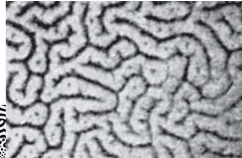
intermediate state of Al plate (type I superconductor)
