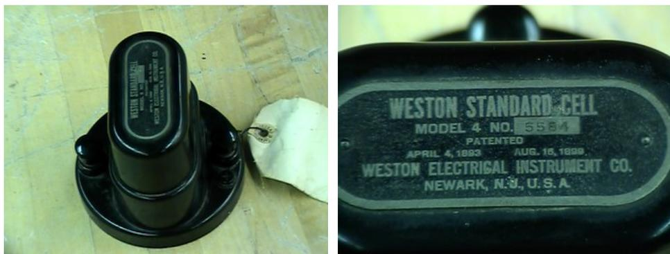
Figure 6.1: The Weston cell. Weston invented and patented the saturated cadmium cell in 1893. It had the advantage of being less temperature sensitive than the previous standard, the Clark cell. It also had the advantage of producing a voltage very near to one volt: 1.0183 V.
