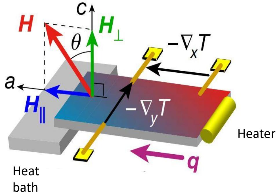
2. Measurement of thermal conductance
