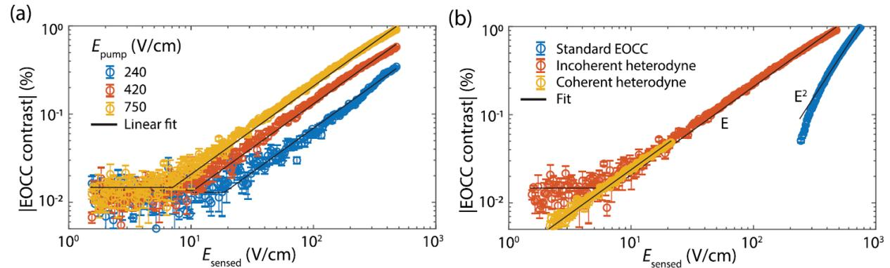
Figure: a) Effect of pump field  $E_{\text{pump}}$ ; b) Quadratic EOCC response vs. (in)coherent heterodyne.
