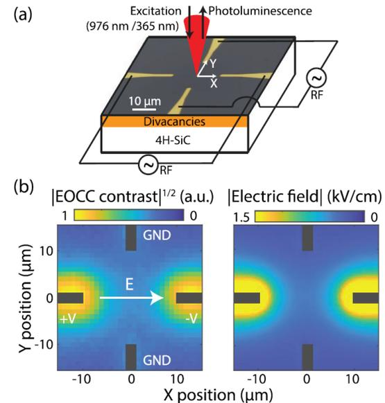
Figure: a) Experimental setup of the sensor b) Measurement (left) and simulation (right).
