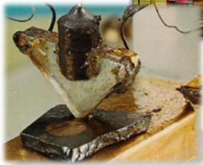
First transistor (1947) Bardeen, Brattain, & Shockley
