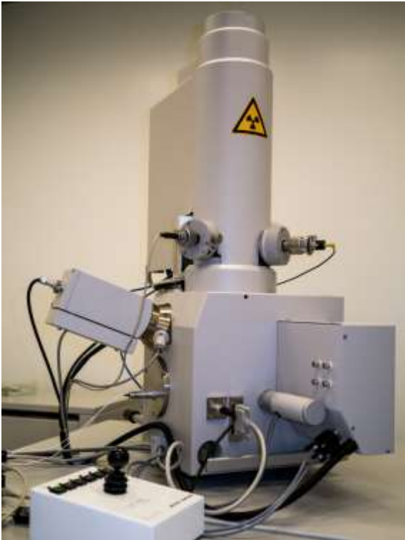
Old WMI EBL system: Philipps scanning electron microscope (SEM) XL30sFEG extended with a Raith laser stage
