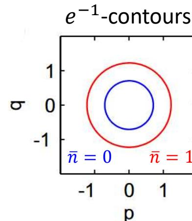
Thermal state  $\hat{\rho}_{\text{th}}$  with  $\bar{n} \equiv \text{Tr}[\hat{a}^\dagger \hat{a} \hat{\rho}_{\text{th}}] = 1$
