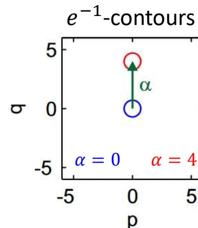
Coherent state  $|\alpha\rangle \equiv |Q + iP\rangle = \hat{D}(\alpha)|0\rangle$
