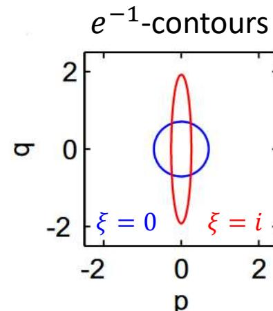
Squeezed vacuum determined by complex squeezing parameter  $\xi \equiv re^{i\varphi}$
