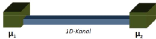
$$I = \frac{e^2}{h} U \quad \text{mit} \quad R_K = \frac{1}{G_K} = \frac{h}{e^2} = 25\,812.807\,4555(59) \, \Omega$$
