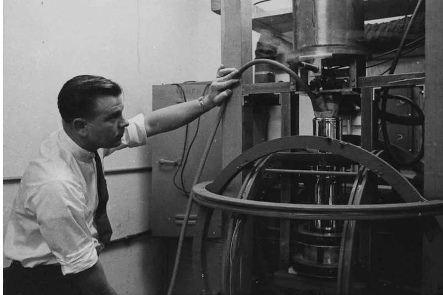
**Measuring the flux quantum.** Graduate student Bascom Deaver refills his apparatus with liquid nitrogen at Stanford University in 1961, a necessary step in maintaining a superconductor at liquid helium temperature. He and William Fairbank used this setup to show that the magnetic field threading a superconducting loop is always quantized. [Credit: J. Mercado/Stanford News Service]
