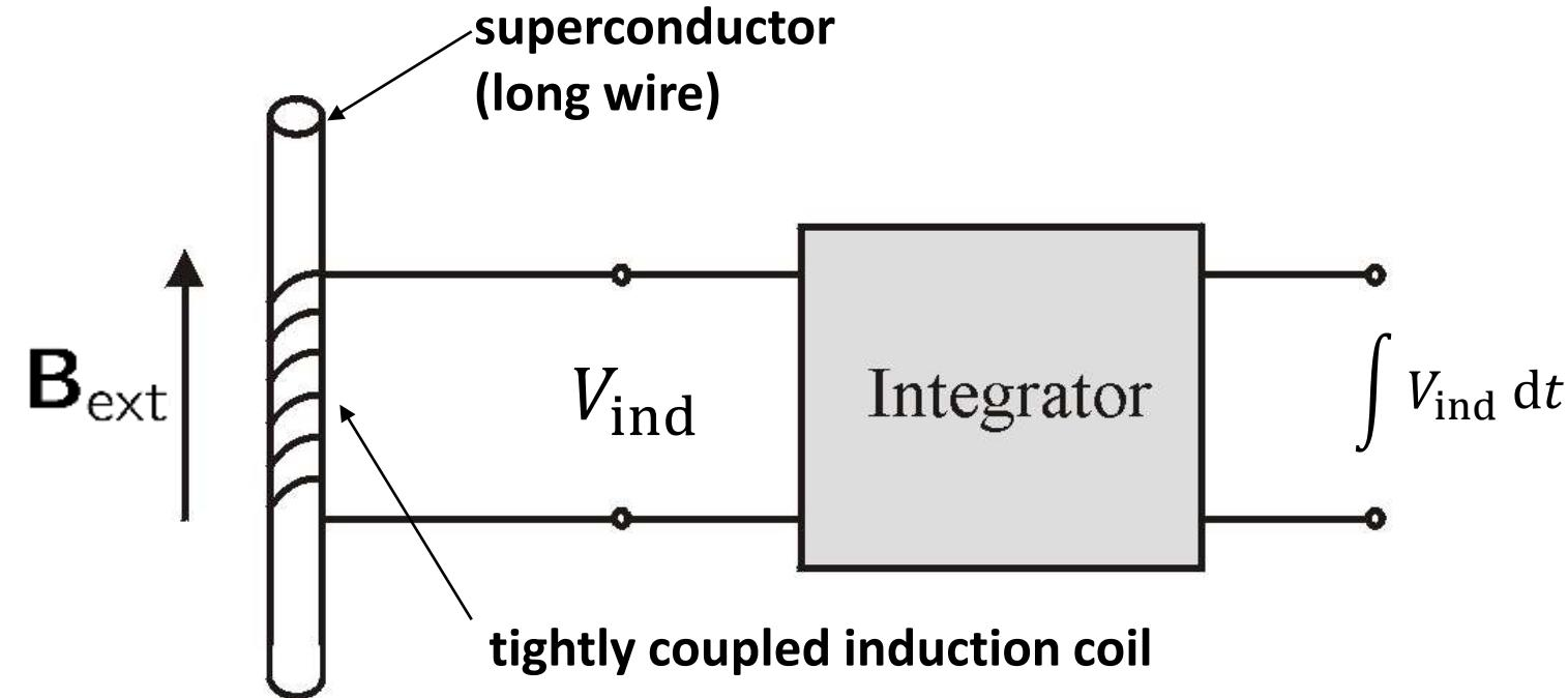
$$V_{\text{ind}} = -\frac{\partial \Phi}{\partial t} \propto -\frac{\partial B_i}{\partial t}$$
