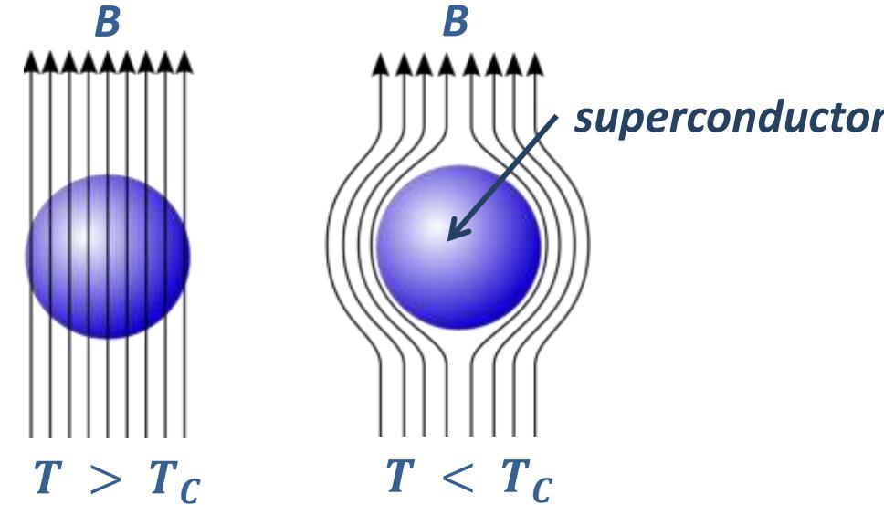
superconductors perfectly expel magnetic field
