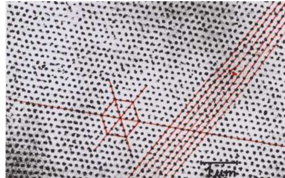
\text{Nb} , T = 4 \text{ K} , disk: 1mm thick, 4 mm \phi B_{\text{ext}} = 985 \text{ G} , a = 170 \text{ nm}
