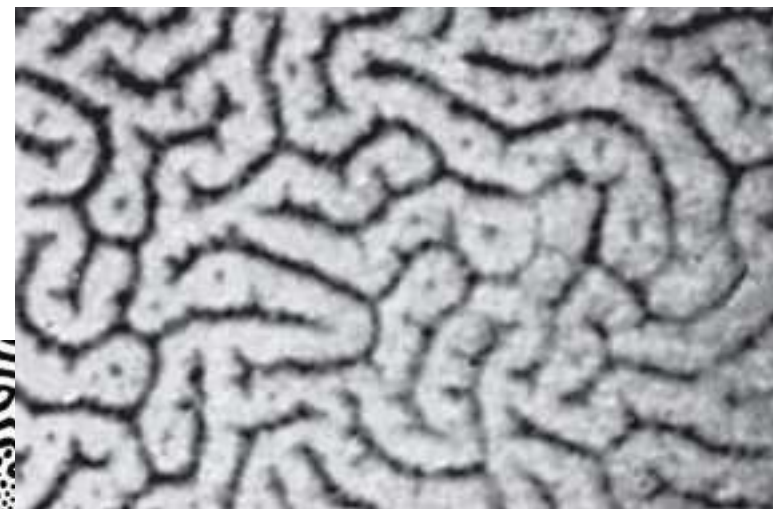
intermediate state of Al plate (type I superconductor)
