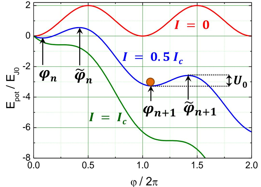
• **junction dynamics: motion of “phase particle”  $\varphi$  in tilted washboard potential** (not discussed here)
