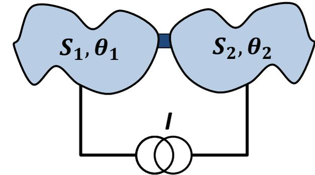
→ Cooper pairs can tunnel through thin insulating barrier ( $T$  = transmission amplitude for single charge carriers)
