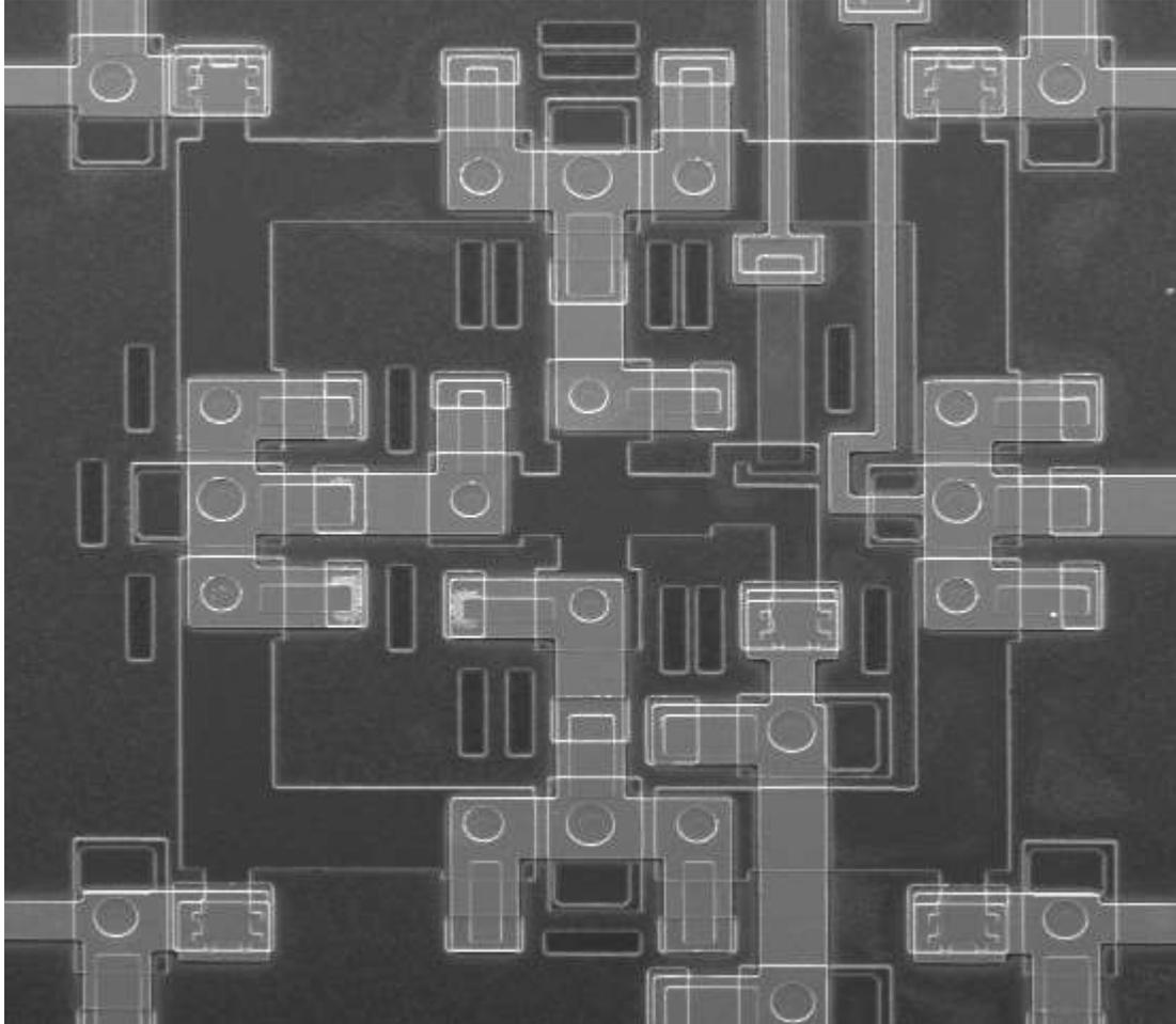
SEM micrograph of a universal asynchronous DR RSFQ (rapid single flux quantum) logic gate
