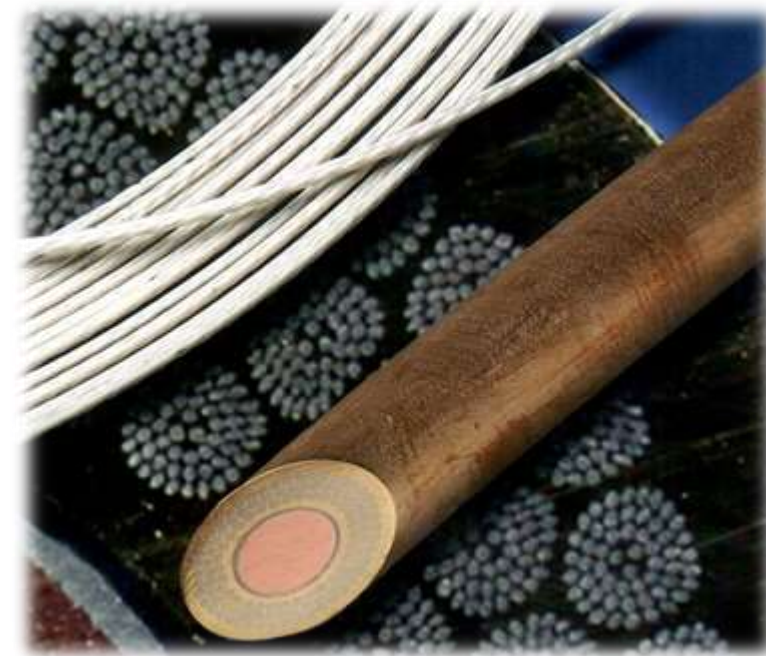
superconducting wires: NbTi, Nb 3 Sn in Cu-matrix
