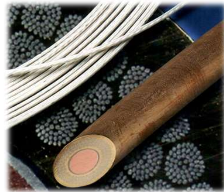
superconducting wires: NbTi, Nb 3 Sn in Cu-matrix
