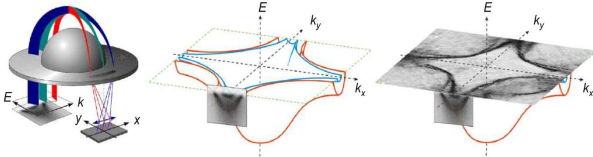
The detector of a modern photoelectron analyzer (left) acts as a **window into the 3D energy-momentum space** of a 2D metal (center). By moving this “window” in  $(\omega, k)$ -space, a full distribution of electrons and its cross-section at the Fermi level — the Fermi surface (right) can be obtained. Shown are the electronic structure and spectra of high-temperature superconductor Bi-2212.
