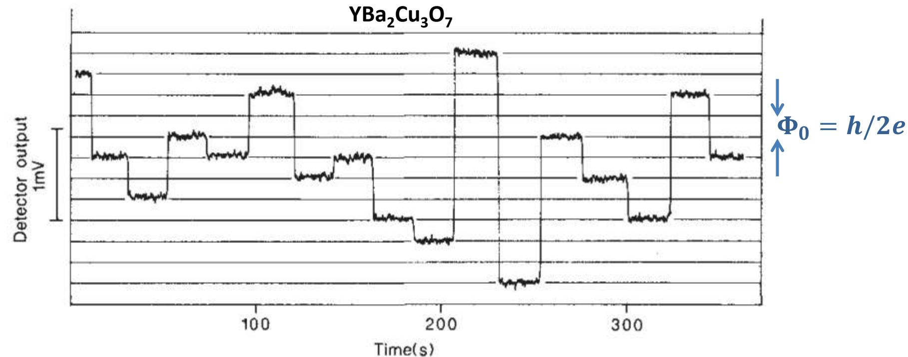
detection of flux jumps with height  $n \cdot \Phi_0 = n \cdot \frac{h}{2e}$
