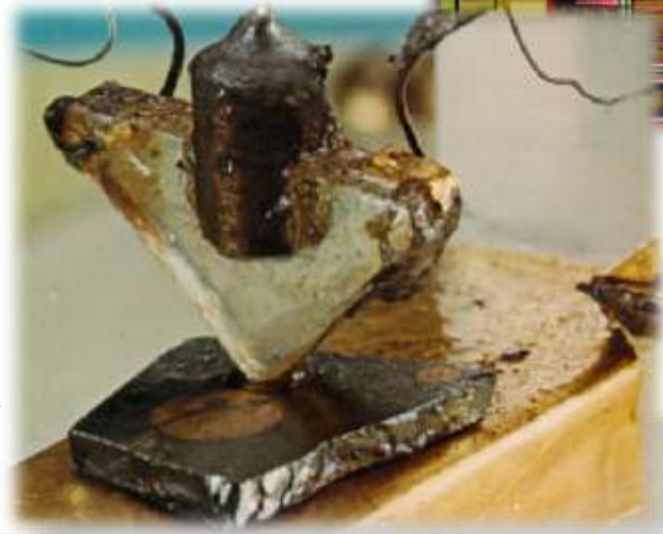
first transistor (1947) Bardeen, Brattain, & Shockley
