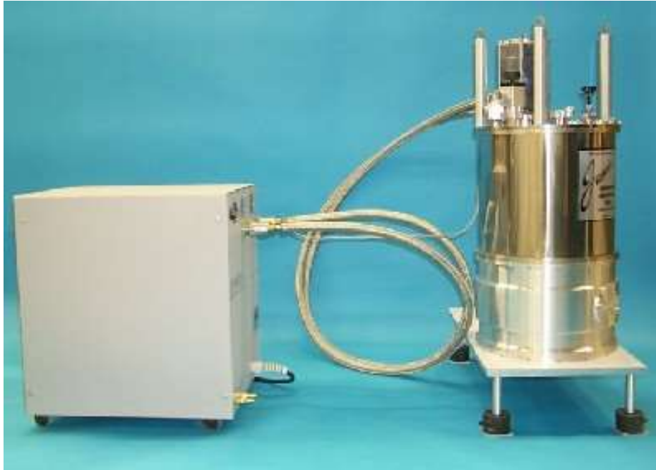
Cryogen-free Two Stage Adiabatic Demagnetization Refrigerator from Janis
