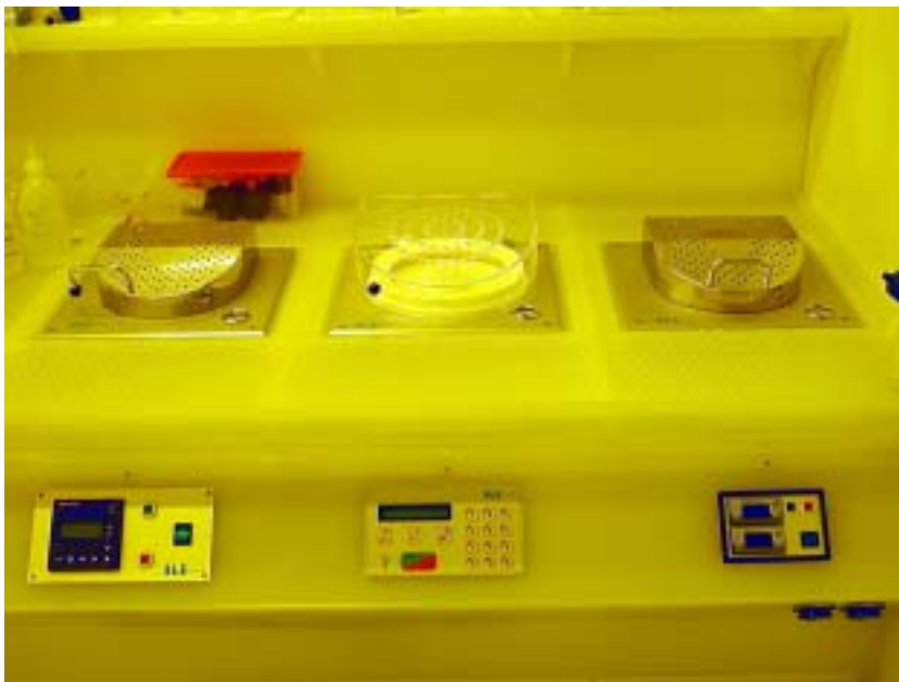
Figure 6: Top: Part of the clean room facility with optical lithography equipment and clean room benches. Bottom: Resist coater and hot plates.
