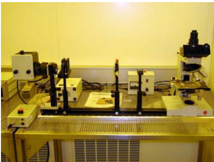
Figure 8: Top: Süss MJB 3 maskaligner for optical lithography. Bottom: Optical projection lithography based on an optical microscope.
