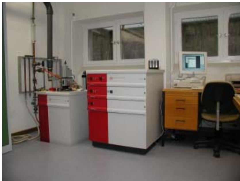
Figure 4: Quantum Design SQUID magnetometer.
