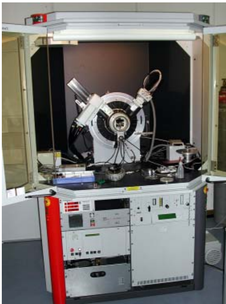
Figure 2: Two-circle X-ray diffractometer Bruker D8 Advance.
