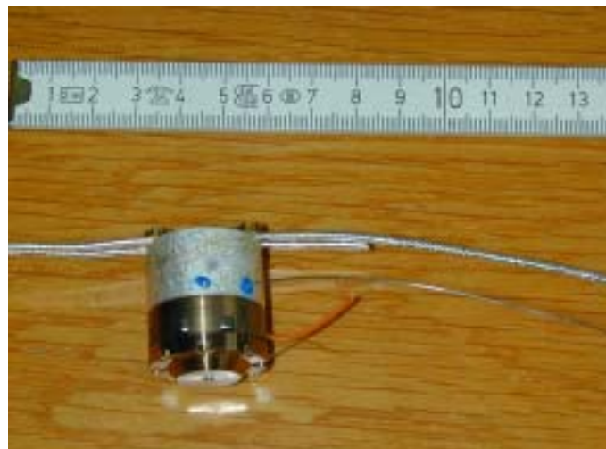
Fig. 3: Experimental cell used to cool solid ^3\text{He} in a silver sinter with an internal NMR coil.
