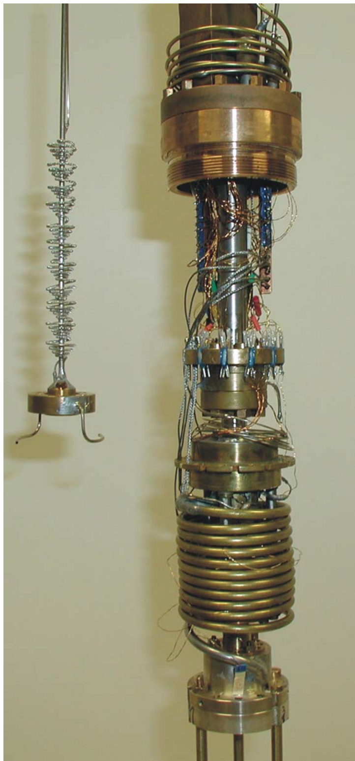
Figure 15: Dilution refrigerator insert with the Joule-Thompson stage, the heat exchanger and the mixing chamber.
