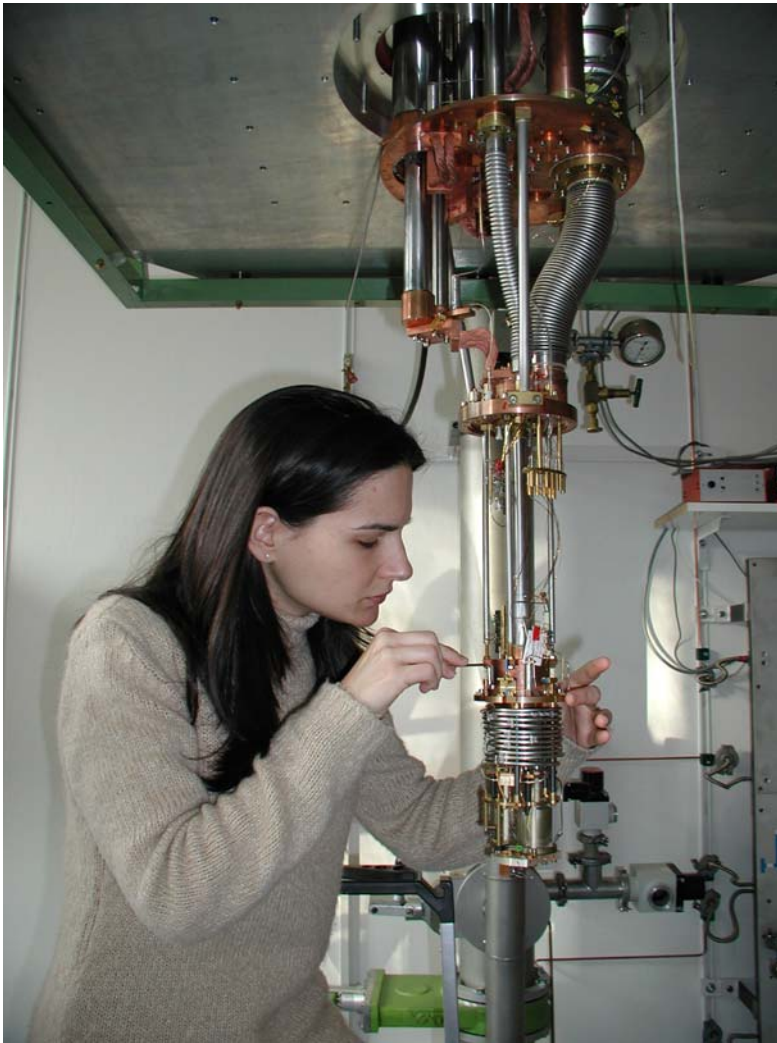
Figure 14: A “dry” millikelvin cooler: dilution refrigerator with pulse-tube pre-cooling.
