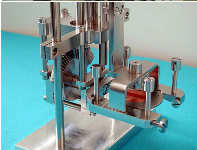
Figure 1: Top: UHV-Laser-Molecular Beam Epitaxy System. Bottom: Sample holder for metallization chamber allowing for evaporation under different angles.
