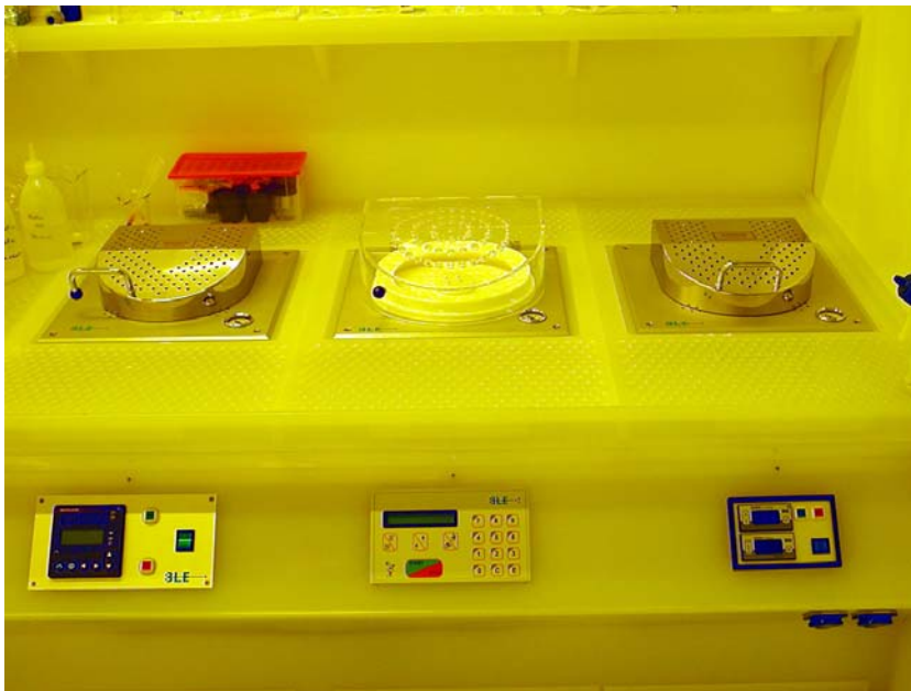
Figure 10: Top: Part of the clean room facility with optical lithography equipment and clean room benches. Bottom: Resist coater and hot plates.
