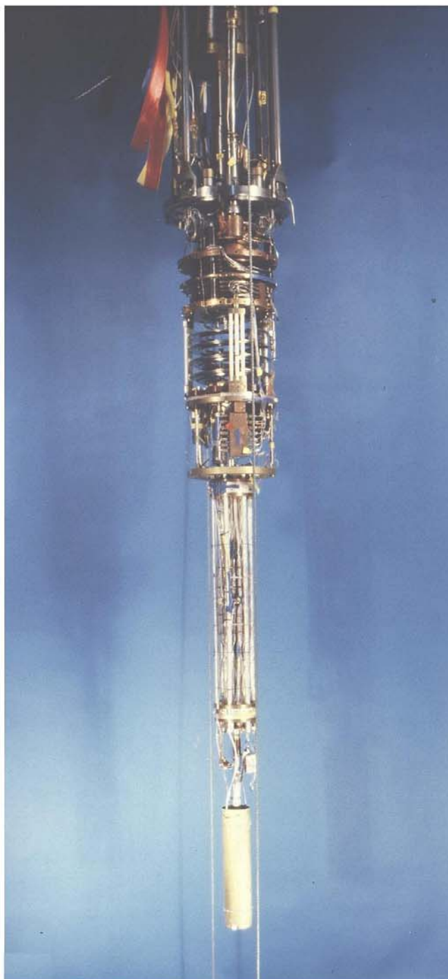
Figure 13: The dilution refrigerator and the nuclear demagnetization stage of the nuclear demagnetization cryostat "Bayerische Millimühle 2".
