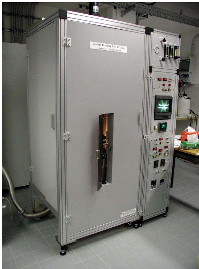
Figure 4: The four-mirror image furnace installed at the crystal laboratory of the WMI. Crystals can be grown by the floating zone and traveling solvent floating zone technique at temperatures up to 2200°C and pressures up to 10 bar.
