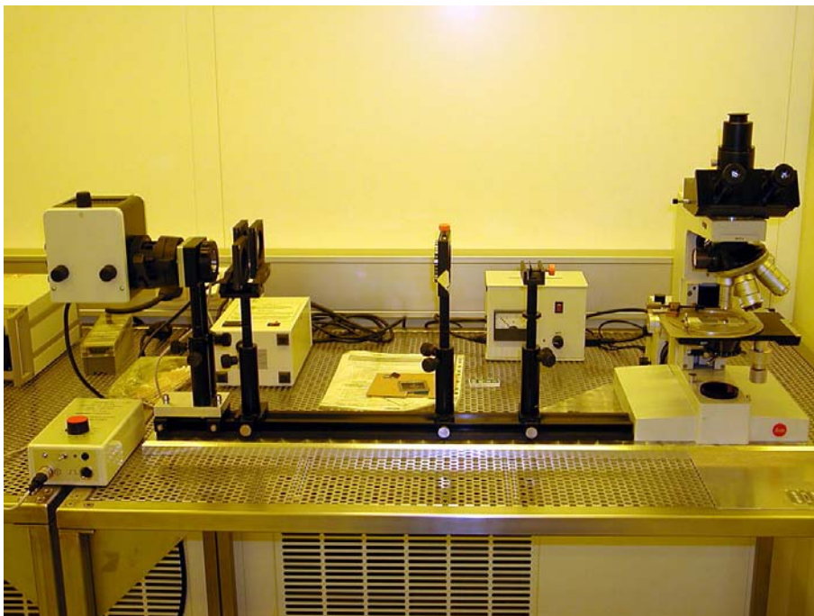
Figure 12: Top: Süss MJB 3 maskaligner for optical lithography. Bottom: Optical projection lithography based on an optical microscope.
