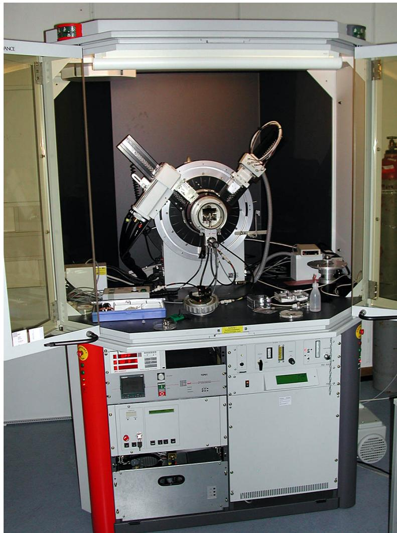
Figure 6: The two-circle X-ray diffractometer Bruker D8 Advance.
