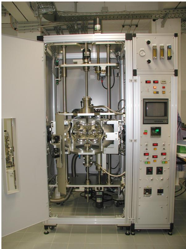
**Figure 2:** The 4-mirror image furnace at the WMI. The maximum temperature is approximately 2200°C at a pressure up to 10 bar. Surfaces required for the various surface sensitive spectroscopies (angle resolved photoemission, Raman and infrared spectroscopy) can be prepared conveniently.
