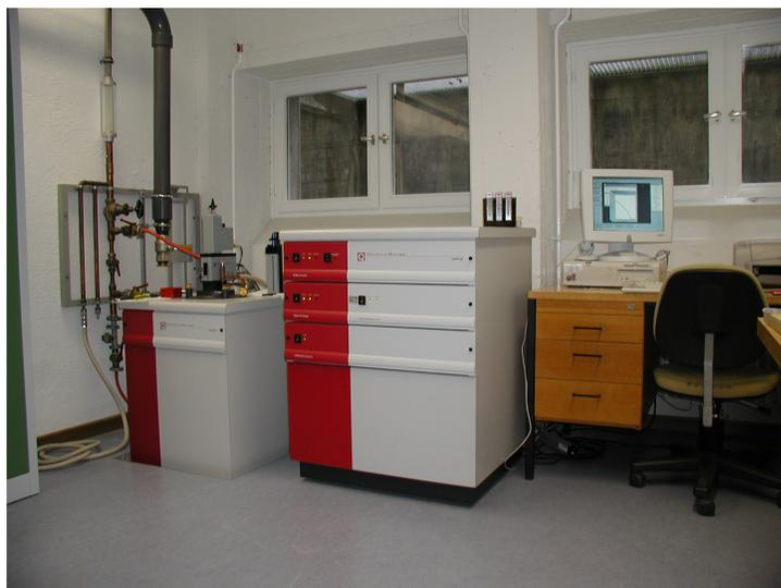
Figure 8: Quantum Design SQUID magnetometer.
