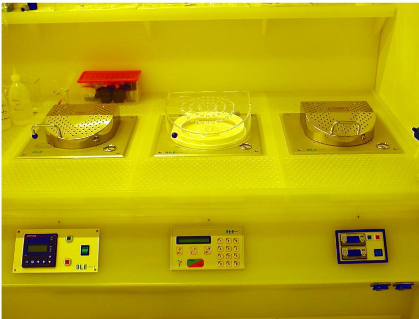
**Figure 10:** Top: Part of the clean room facility with optical lithography equipment and clean room benches. Bottom: Resist coater and hot plates.
