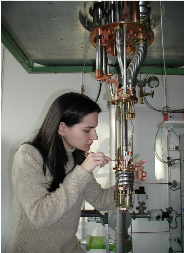
**Figure 14:** A “dry” millikelvin cooler: dilution refrigerator with pulse-tube pre-cooling developed at WMI.
