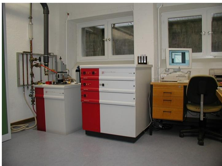
Figure 8: Quantum Design SQUID magnetometer.
