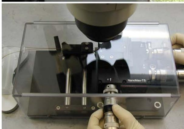
realized by inserting the cantilevers into an array of liquid-filled micro capillaries in a functionalization unit. The process of chemical functionalization then takes place within minutes or hours controlled through a high resolution optical microscope by a camera.
