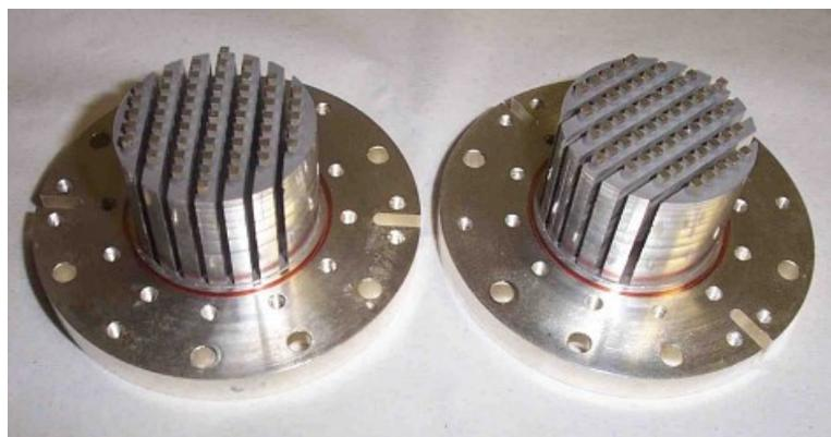
**Figure 16:** Two mixing chamber mounting plates with silver sponges. Those are needed to overcome the thermal resistance (Kapitza resistance) between the liquid  $^3\text{He}$  and the mounting plate of the mixing chamber. To fabricate the mounting of the sponge (square pins embedded in the sponge) a spark erosion technique has been employed.
