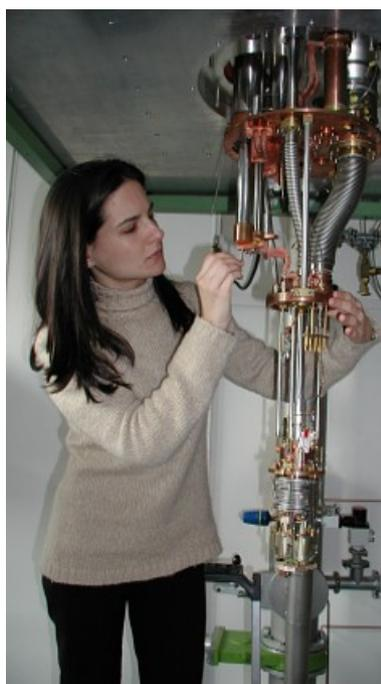
**Figure 14:** The "dry" dilution refrigerator of the WMI.
