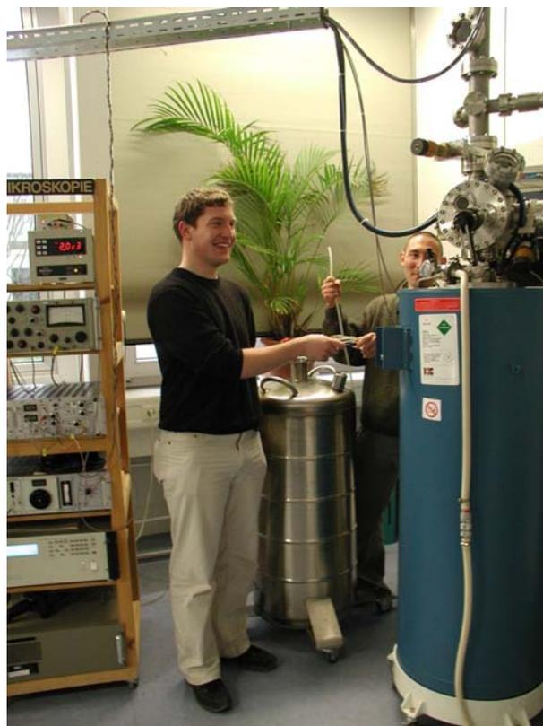
The STM is optimized for low temperature tunneling imaging and spectroscopy in high magnetic fields under UHV-conditions (see picture: STM in the cryostat). A self-built electronics allows scanning tunneling spectroscopy at points along lines, in grids and in a high density mode.
