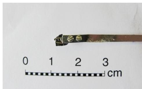
**Figure 1:** The largest sample of  $\text{YbRh}_2\text{Si}_2$  used in this work mounted in a 5N Ag clamp.
