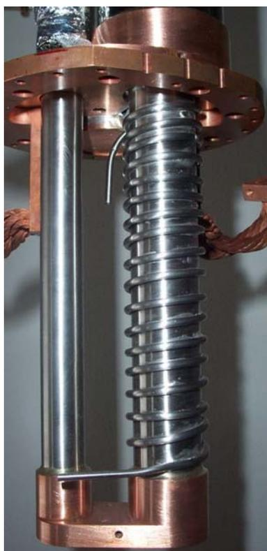
**Figure 4:** Lower half of our PTR. At the top of the photo is its first stage, at the bottom the second stage, and in between the second pulse tube and the regenerator with the hex made from a stainless steel capillary.
