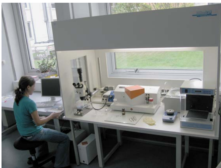
Figure 24: Clean environment (bio) work bench: Cantilever setup and cell-handling equipment inside the laminar flow box.
