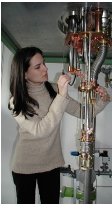
Figure 14: The "dry" dilution refrigerator of the WMI.
