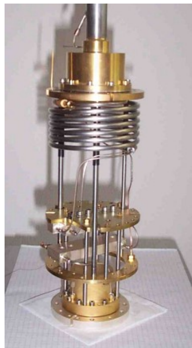
Figure 15: Low-temperature unit of a WMI dilution refrigerator ready to go into a cryostat.
