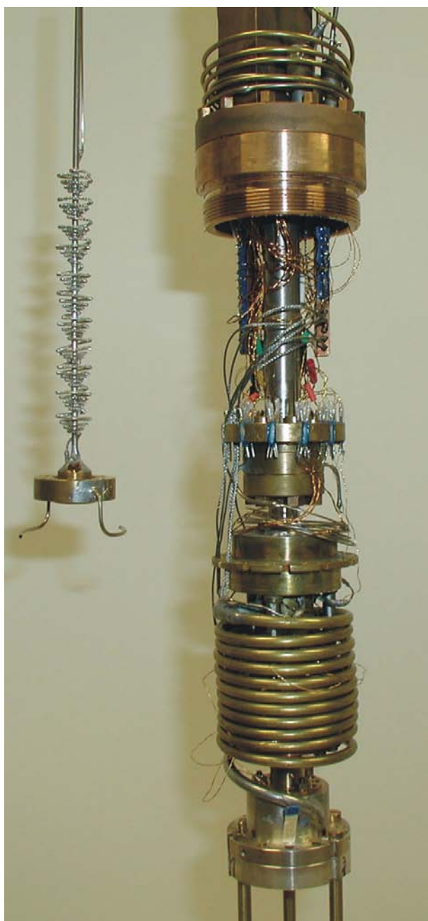
Figure 17: Dilution refrigerator insert with the Joule-Thompson stage, the heat exchanger and the mixing chamber.
