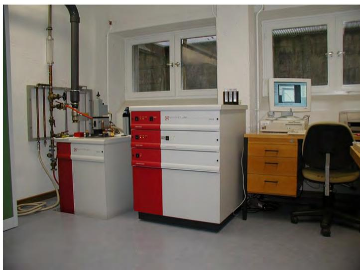
Figure 8: Quantum Design SQUID magnetometer.
