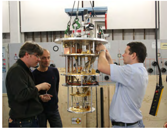
Figure 1: Unpacking the dilution unit. The dilution unit hanging from the crane and still protected by the aluminium frame with is in the process to be removed.
