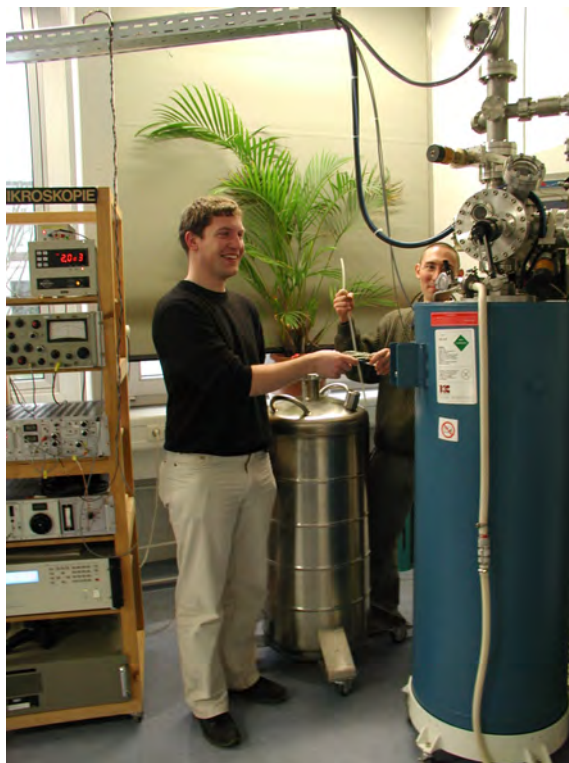
Figure 19: The current setup of the instrument: visible is the cryostat with microscope inside, as well as parts of the control electronics.
