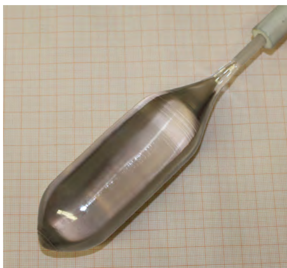
Figure 2: \text{CaWO}_4 crystal of 886 g with seed holder and seed after growth. The slightly grey colour of the crystal is due to an oxygen deficiency originating from the low oxygen partial pressure in the growth atmosphere. The grey colour can be removed by a subsequent annealing procedure in pure oxygen at elevated temperatures.
