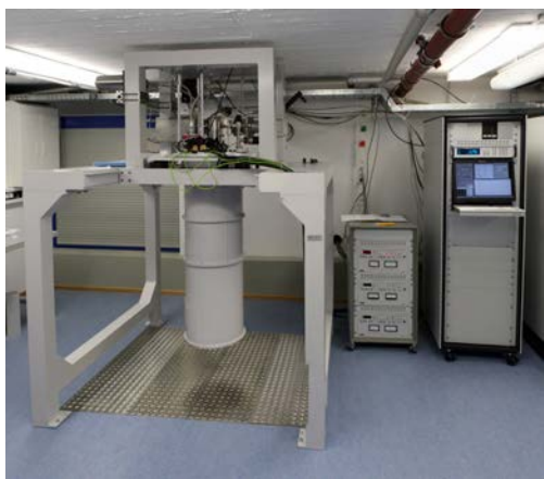
Figure 17: The dilution system with the 3D vector magnet located in the Quantum Laboratories and operating at base-temperature.
