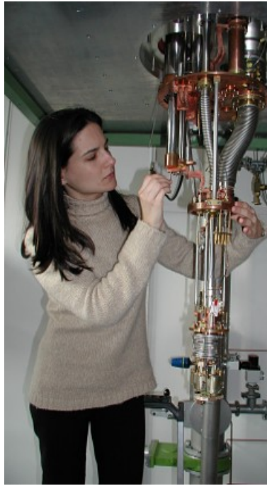
Figure 14: The "dry" dilution refrigerator of the WMI.
