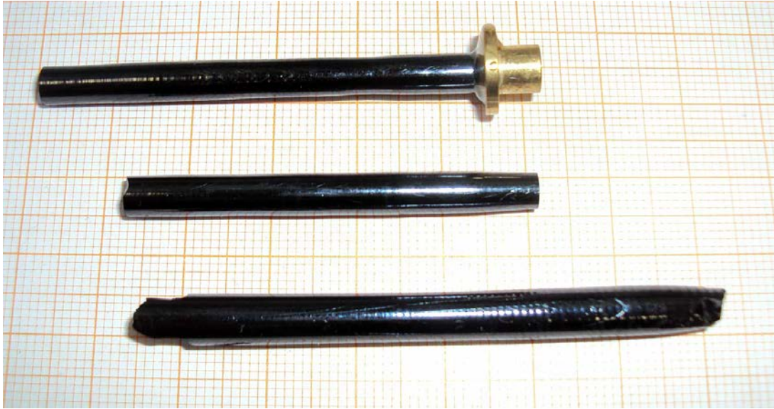
Figure 2: Y 3 Fe 5 O 12 single crystals grown by the TSFZ method. With growth speeds up to 4 mm/h this method is quite effective to produce large single crystals of this compound.
