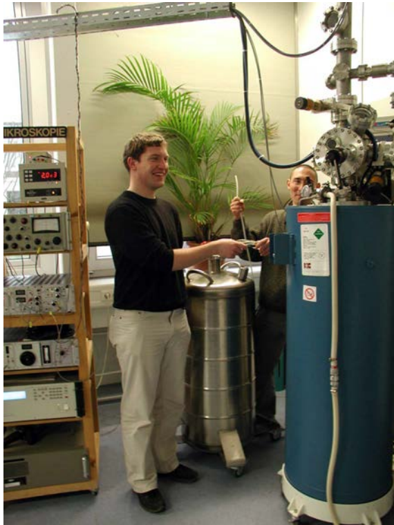
Figure 21: The current setup of the instrument: visible is the cryostat with microscope inside, as well as parts of the control electronics.
