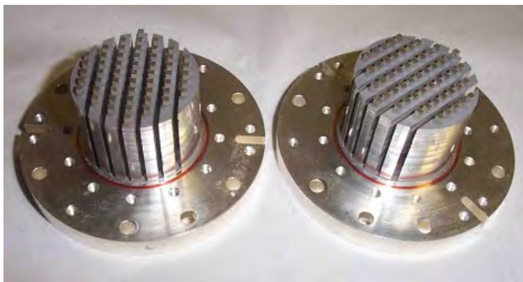
Figure 16: Two mixing chamber mounting plates with silver sponges. Those are needed to overcome the thermal resistance (Kapitza resistance) between the liquid ^3\text{He} and the mounting plate of the mixing chamber. To fabricate the mounting of the sponge (square pins embedded in the sponge) a spark erosion technique has been employed.
