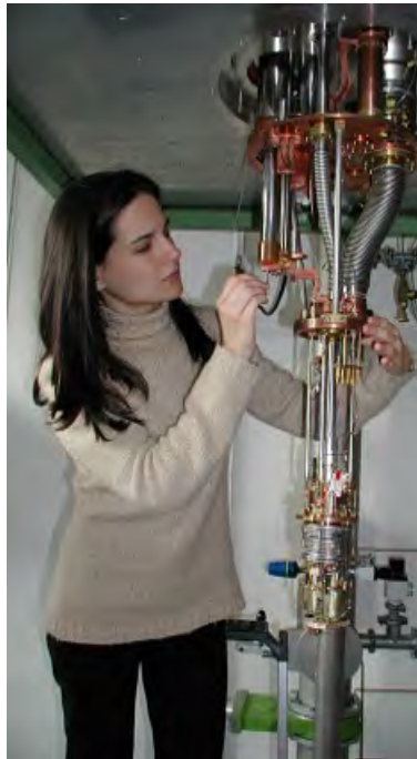
Figure 14: The "dry" dilution refrigerator of the WMI.
