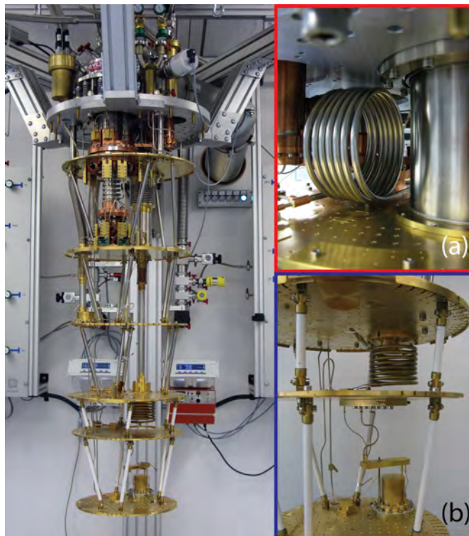
Figure 1: Photographs of the fully operational new cryogen-free dilution refrigerator. (a) Improved counterflow heat exchanger in the ^4\text{He} precooling circuit. In (b) the concentric tube and two step heat exchangers as well as the mixing chamber can be seen from top to bottom.
