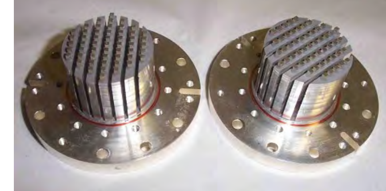
Figure 17: Two mixing chamber mounting plates with silver sponges. Those are needed to overcome the thermal resistance (Kapitza resistance) between the liquid {}^3\text{He} and the mounting plate of the mixing chamber. To fabricate the mounting of the sponge (square pins embedded in the sponge) a spark erosion technique has been employed.
