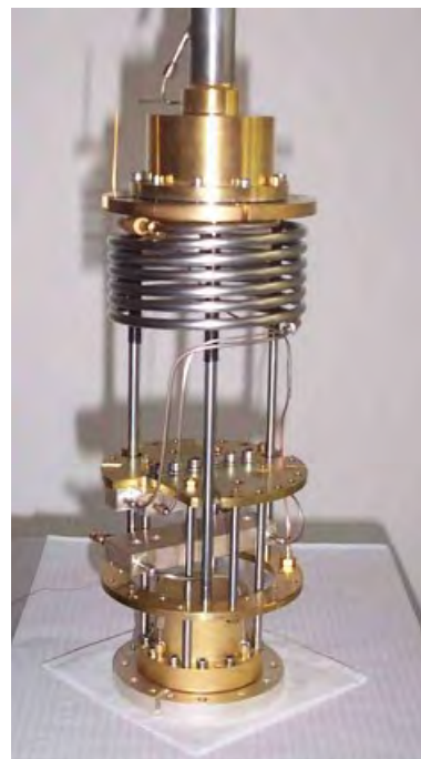
Figure 16: Low-temperature unit of a WMI dilution refrigerator ready to go into a cryostat.
