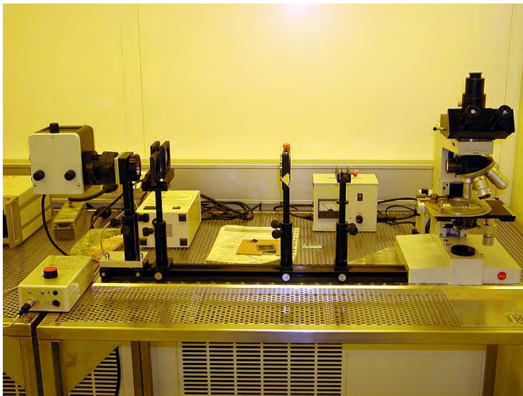
Figure 14: Top: Süss MJB 3 maskaligner for optical lithography. Bottom: Optical projection lithography based on an optical microscope.
