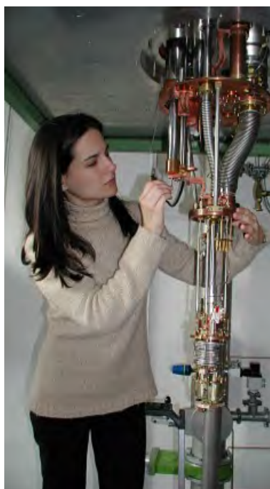
Figure 17: The "dry" dilution refrigerator of the WMI.
