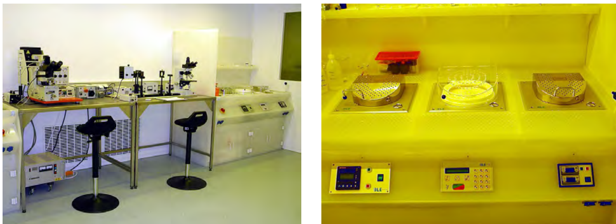
Figure 12: Top: Part of the clean room facility with optical lithography equipment and clean room benches. Bottom: Resist coater and hot plates.
