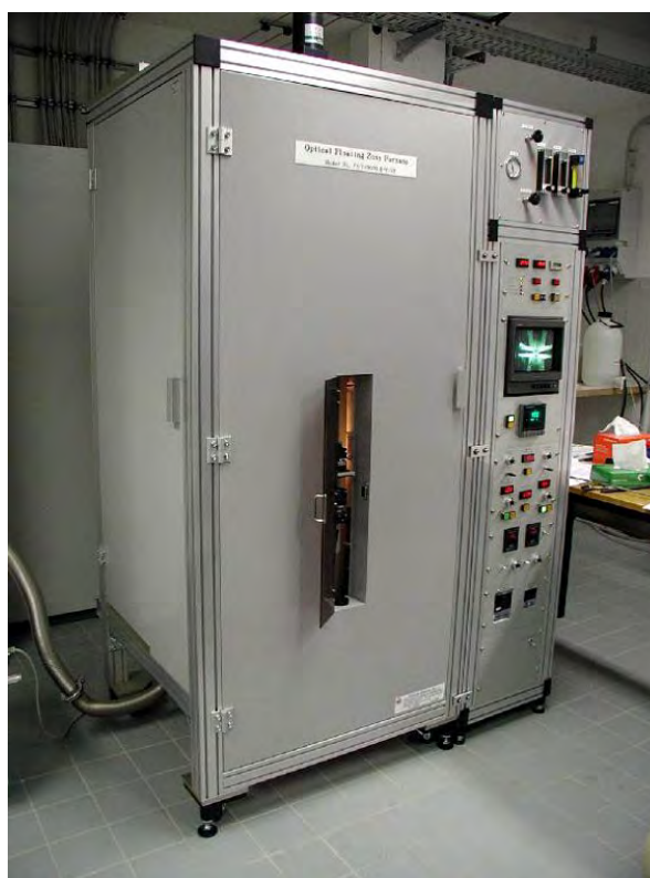
Figure 5: The four-mirror image furnace installed at the crystal laboratory of the WMI. Crystals can be grown by the floating zone and traveling solvent floating zone techniques at temperatures up to 2200 °C and pressures up to 10 bar.
