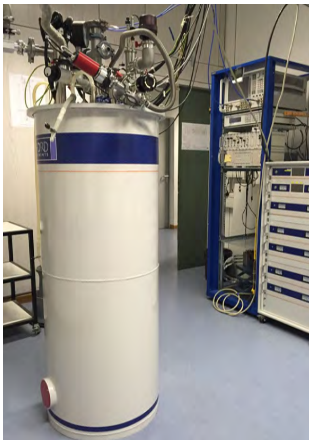
Figure 11: The 3D vector magnet with control electronics in the “CHAOS” Laboratory.
