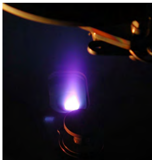
Figure 2: Pulsed Laser Deposition (PLD): When the pulse of the UV laser (KrF excimer laser, 248 nm) hits the target, the target material is ablated and the so-called laser “plume” containing highly excited atoms and molecules is formed.
