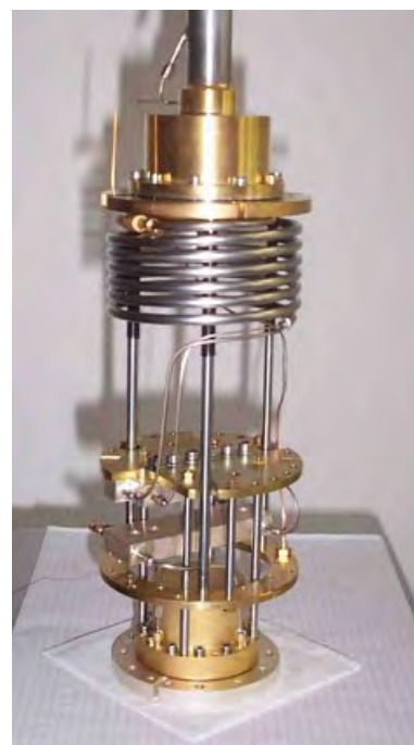
Figure 18: Low-temperature unit of a WMI dilution refrigerator ready to go into a cryostat.
