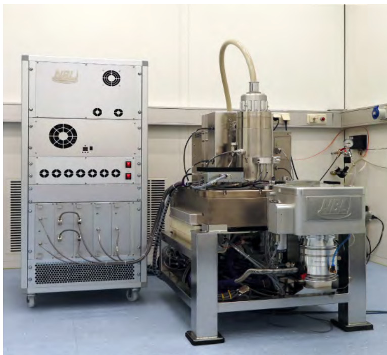
Figure 13: 100 kV Electron Beam Lithography System nB5 of NanoBeam Ltd., UK, inside the WMI cleanroom facility.
