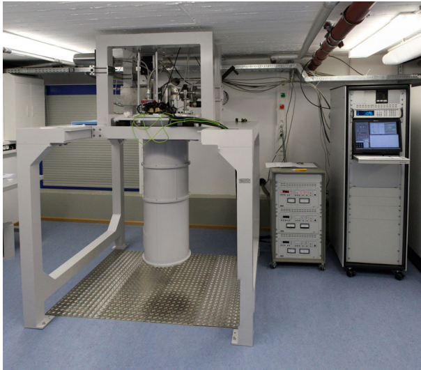
Figure 20: The dilution refrigerator with the 3D vector magnet located in the Quantum Laboratories.
