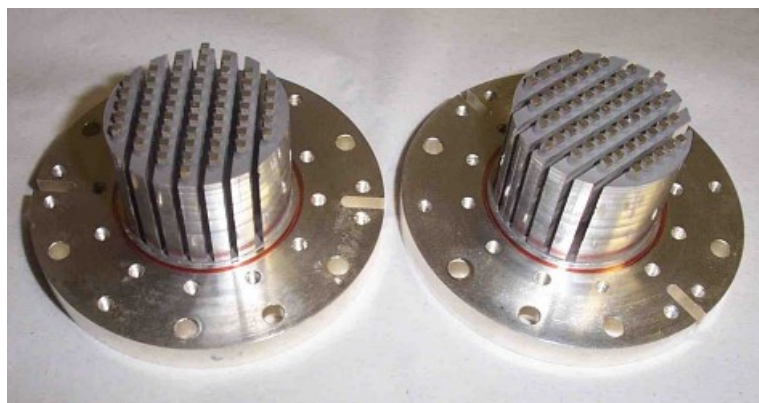
Figure 19: Two mixing chamber mounting plates with silver sponges. Those are needed to overcome the thermal resistance (Kapitza resistance) between the liquid ^3\text{He} and the mounting plate of the mixing chamber. To fabricate the mounting of the sponge (square pins embedded in the sponge) a spark erosion technique has been employed.
