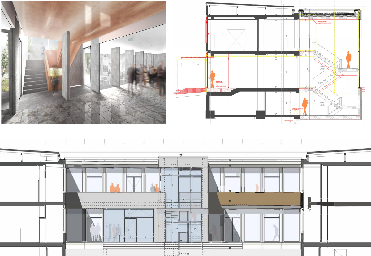
Figure 2: Top left: An artists view of the new main staircase of the WMI building. Top right: Cross-sectional view of the new main staircase. Bottom: View of the cross-aisle and the new stairway as seen from the inner courtyard.
