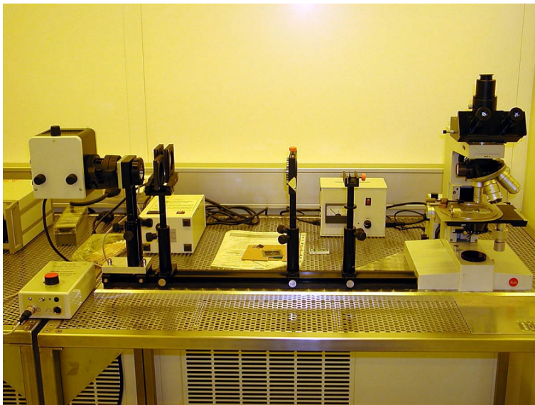
Figure 16: Top: Süss MJB 3 maskaligner for optical lithography. Bottom: Optical projection lithography based on an optical microscope.
