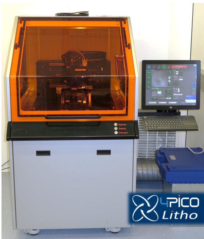
Figure 1: The direct laser writing system PicoMaster 200 installed in the WMI clean room.
