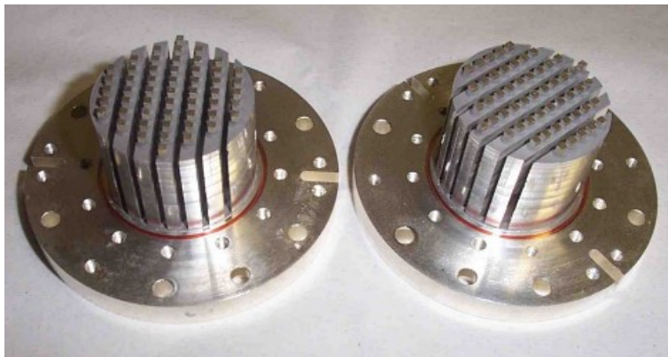
Figure 20: Two mixing chamber mounting plates with silver sponges. Those are needed to overcome the thermal resistance (Kapitza resistance) between the liquid ^3\text{He} and the mounting plate of the mixing chamber. To fabricate the mounting of the sponge (square pins embedded in the sponge) a spark erosion technique has been employed.
