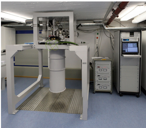
Figure 21: The dilution refrigerator with the 3D vector magnet located in the Quantum Laboratories.
