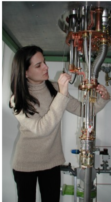
Figure 18: The "dry" dilution refrigerator of the WMI.
