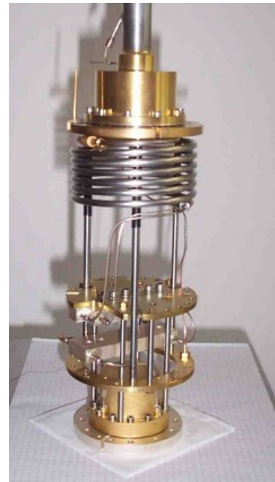
Figure 19: Low-temperature unit of a WMI dilution refrigerator ready to go into a cryostat.
