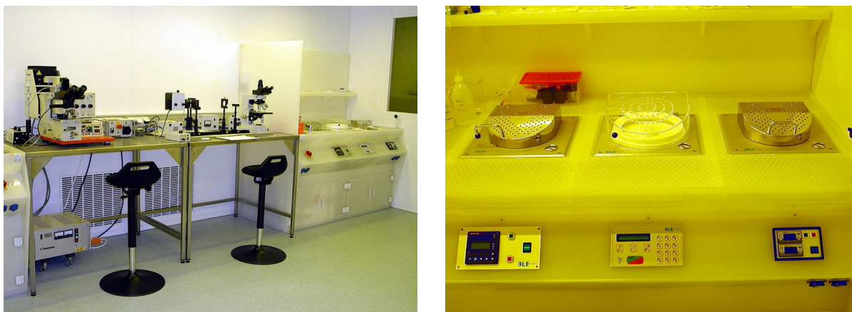
Figure 13: Top: Part of the clean room facility with optical lithography equipment and clean room benches. Bottom: Resist coater and hot plates.
