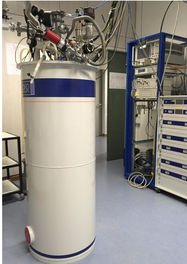
Figure 12: The 3D vector magnet with control electronics in the “CHAOS” Laboratory.
