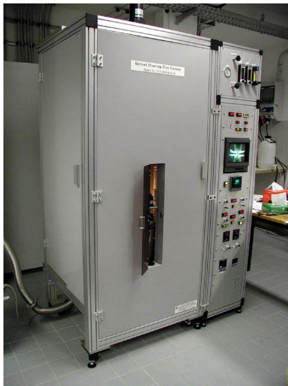
Figure 6: The four-mirror image furnace installed at the crystal laboratory of the WMI. Crystals can be grown by the floating zone and traveling solvent floating zone techniques at temperatures up to 2200 °C and pressures up to 10 bar.
