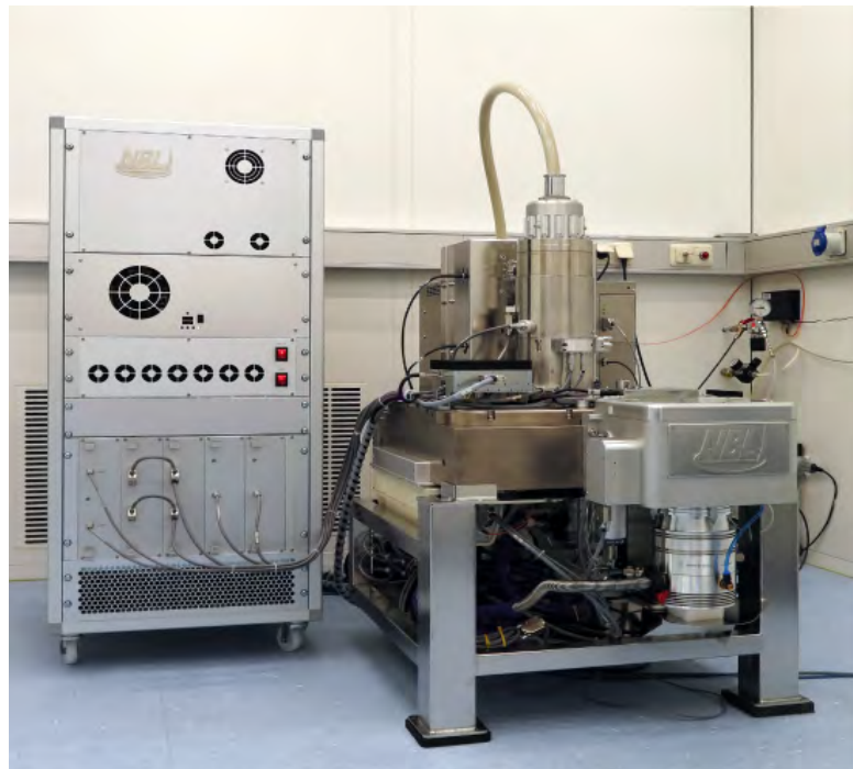
Figure 15: 100 kV Electron Beam Lithography System nB5 of NanoBeam Ltd., UK, inside the WMI cleanroom facility.
