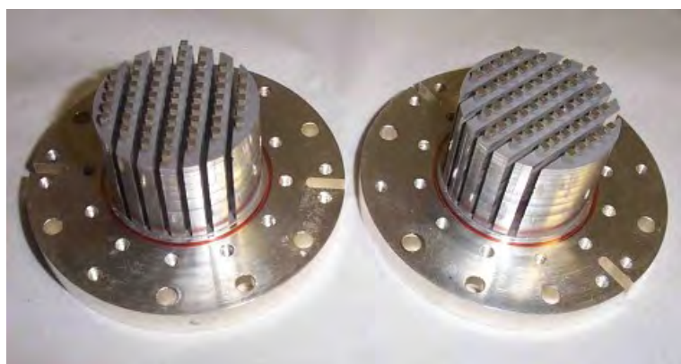
Figure 21: Two mixing chamber mounting plates with silver sponges. Those are needed to overcome the thermal resistance (Kapitza resistance) between the liquid ^3\text{He} and the mounting plate of the mixing chamber. To fabricate the mounting of the sponge (square pins embedded in the sponge) a spark erosion technique has been employed.
