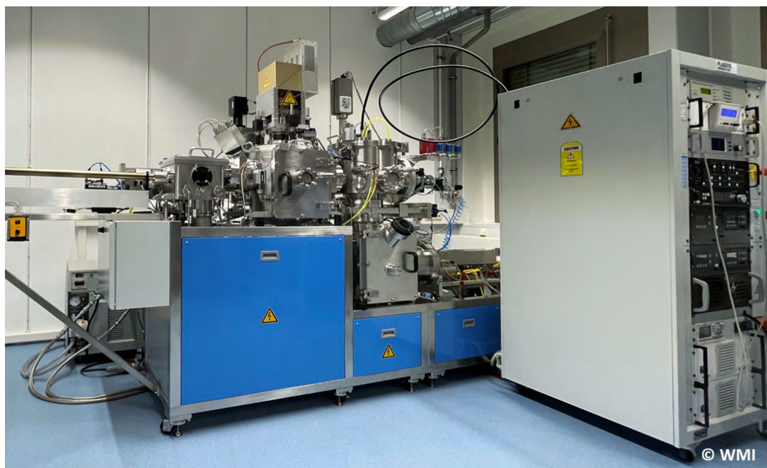
Figure 1: The Plassys UHV deposition system installed at WMI. Left part: loadlock with the sample transfer rod, middle part: sputter deposition chamber, right part: deposition/oxidation and electron beam evaporation chambers. The deposition/oxidation chamber is positioned atop the evaporation chamber separated by a horizontal gate valve. Not shown is the computer system for process control.
