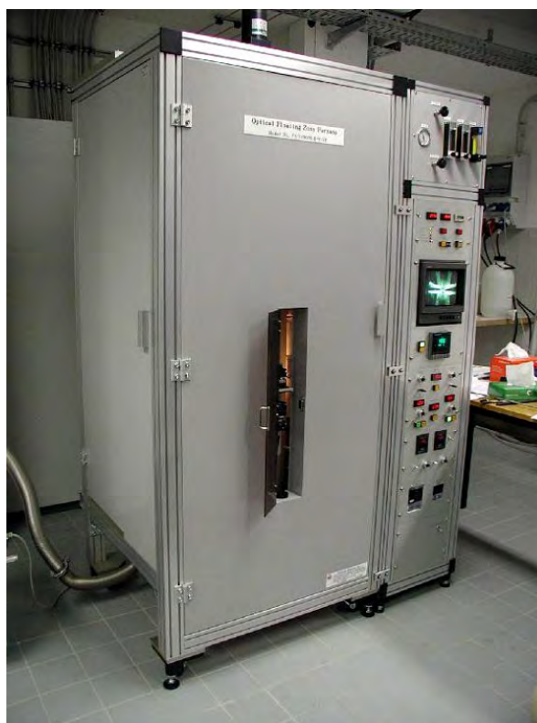
Figure 7: The four-mirror image furnace installed at the crystal laboratory of the WMI. Crystals can be grown by the floating zone and traveling solvent floating zone techniques at temperatures up to 2200 °C and pressures up to 10 bar.
