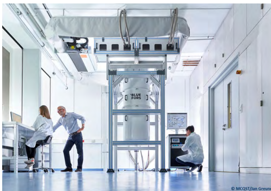
Figure 1: New Bluefors XLD 1000 Dry Dilution Refrigerator after installation at WMI. All the compressors and the gas handling systems are located in a technical room underneath the laboratory (photo: MCQST/Jan Greune).
