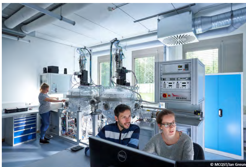
Figure 4: UHV sputter deposition system named «SUPERBOWLS». Left chamber is the NFC dedicated to the deposition of superconducting materials, right chamber is the AFC equipped with magnetic materials. Between the two deposition chambers resides the loadlock (LL).
