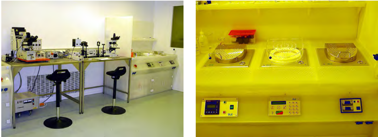
Figure 14: Top: Part of the clean room facility with optical lithography equipment and clean room benches. Bottom: Resist coater and hot plates.
