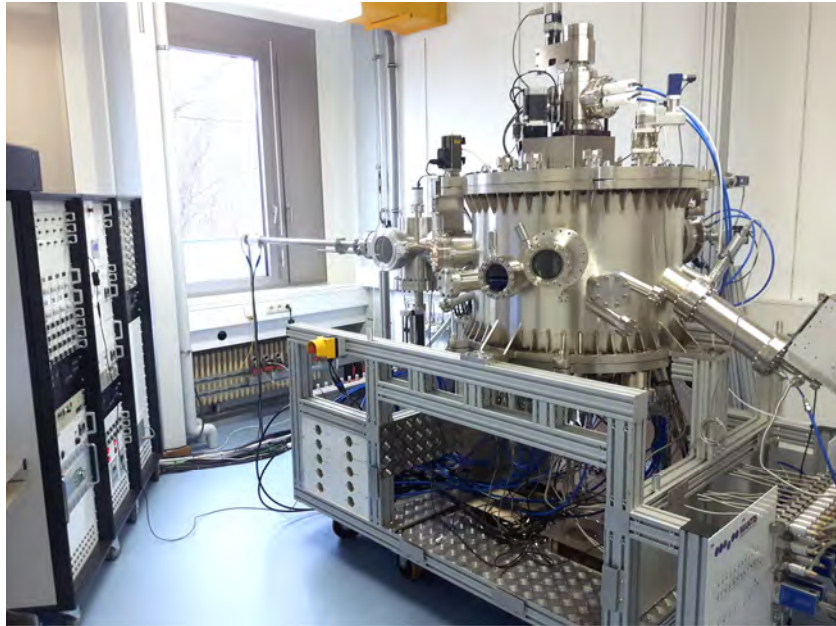
Figure 5: UHV sputter deposition system named «ULTRADISC». The main chamber contains the deposition sources in the bottom flange and the substrate manipulator on the top flange.
