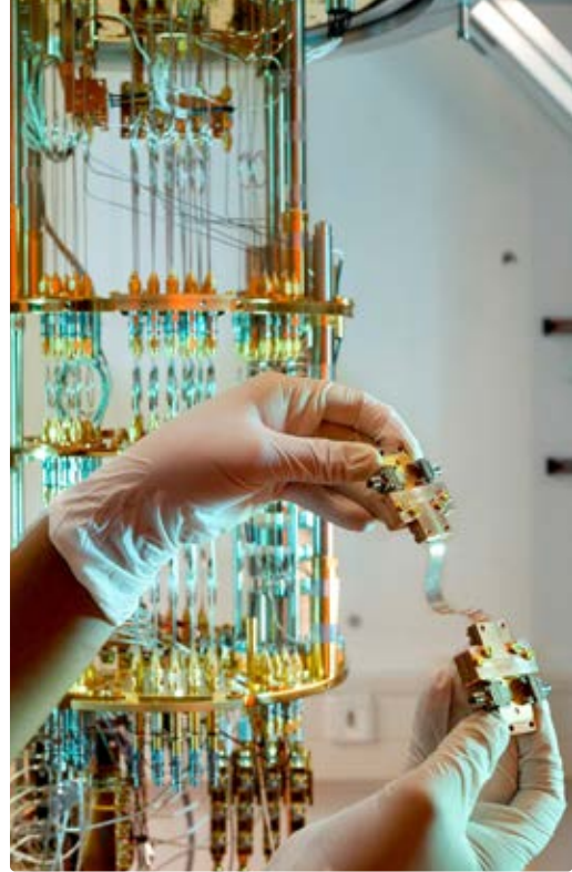
A flexible superconducting cable interfacing two microwave connectors.
