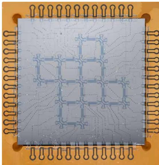
The 17-qubit chip fabricated and operated in the laboratories of WMI. Fixed-frequency qubits (cross-shaped) are linked by tunable couplers (edges) in a shape particular suitable for error correction.
