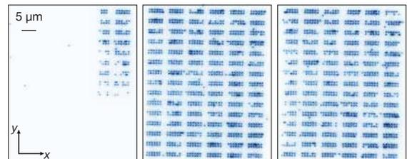
Exemplary single shots at various instances in time of an iteratively assembled array exceeding 1,000 atoms on average. The first image on the left shows the initial gradual loading of the array.
