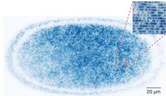
A single-shot image of more than 10,000 single atoms directly loaded into the bow-tie lattice from the magneto-optical trap. The smaller red box is an enlargement which shows well-resolved single atoms.
