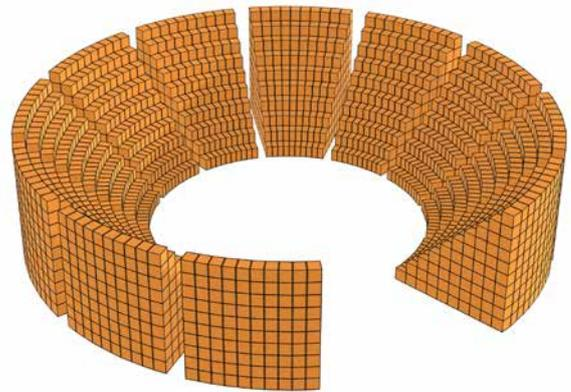
The 3D-local architecture (arrangement of qubits) of the shallow quantum circuit resembles the Colosseum. It is designed to tolerate noise and is appropriate for computation on near-term quantum devices.
