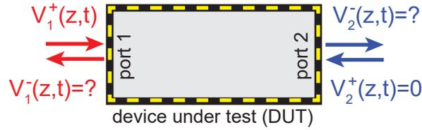
Figure 2.6: In a transmission measurement we apply a well defined signal  $V_1^+(z, t)$  at one defined input port and no signal at the other. Reflection and transmission are measured.
