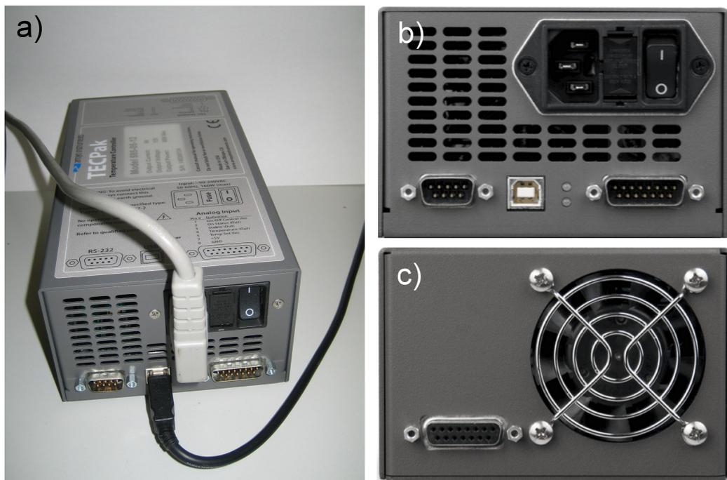
Figure 3.2: TECPak PID controller from Arroyo Instruments. **a)** Front panel with the power cable and the USB connector to the computer. **b)** Front panel with power, USB, RS-232 and analog ports. **c)** Rear panel with one port for the input signal coming from the temperature sensor and the output line for the fans [9].
