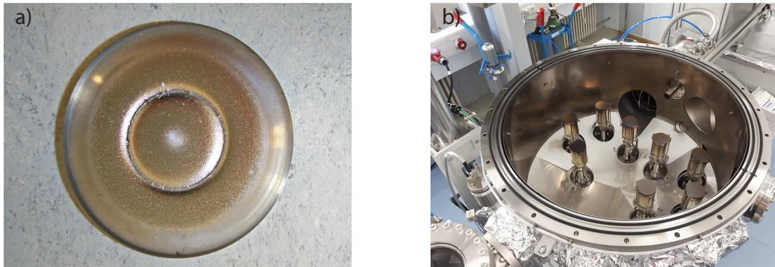
**Figure 2.4:** a) Used  $\text{Co}_{25}\text{Fe}_{75}$  target after several deposition runs and removal from the magnetron. The circular grinding of the material indicates where the electrons were kept gyrating by the magnetic fields. The diameter of the target is 50.8 mm. b) Inside of the SP4 chamber, 8 magnetrons are placed in two deposition clusters for complex multilayer deposition. Both, face-to-face and confocal sputtering is possible with this setup.<sup>2</sup>
