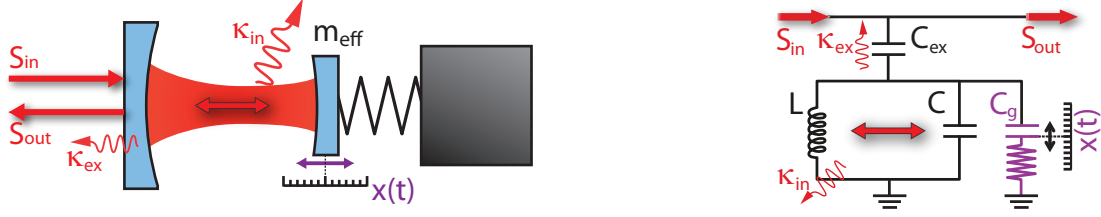
Figure 4.1: Schematic showing an optomechanical system as a single sided Fabry-Perot cavity with one vibrating mirror (left) and an equivalent circuit scheme of an electromechanical system (right). The input and output fields are indicated by S_{\text{in}} and S_{\text{out}} , respectively. The losses into the environment and into the feeds are indicated by \kappa_{\text{in}} and \kappa_{\text{ex}} , respectively. Both systems are described by the same Hamiltonian defined in equation 4.2.
