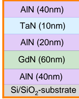
Fig. 6.7: SMR reference sample : FMI AlN/GdN/AlN/TaN/AlN heterostructure on a Si/SiO 2 substrate.
