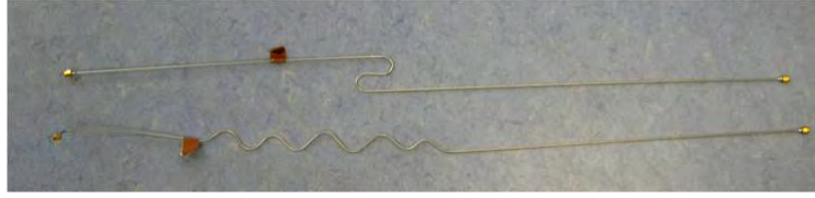
Figure 3.6: Two of the four used semi rigid coaxial cables. The length of each cable is approximate 1 m.
