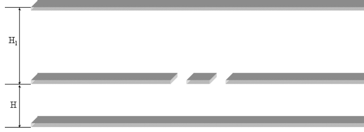
Figure 2.3: Configuration of the air capacitance of a CPW.
