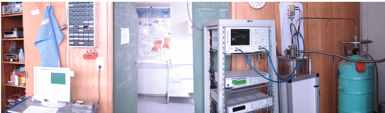
Figure 4.4: Picture of the measurement setup with PC (with LabView) on the left, helium can on the right and RT measurement devices in between.
