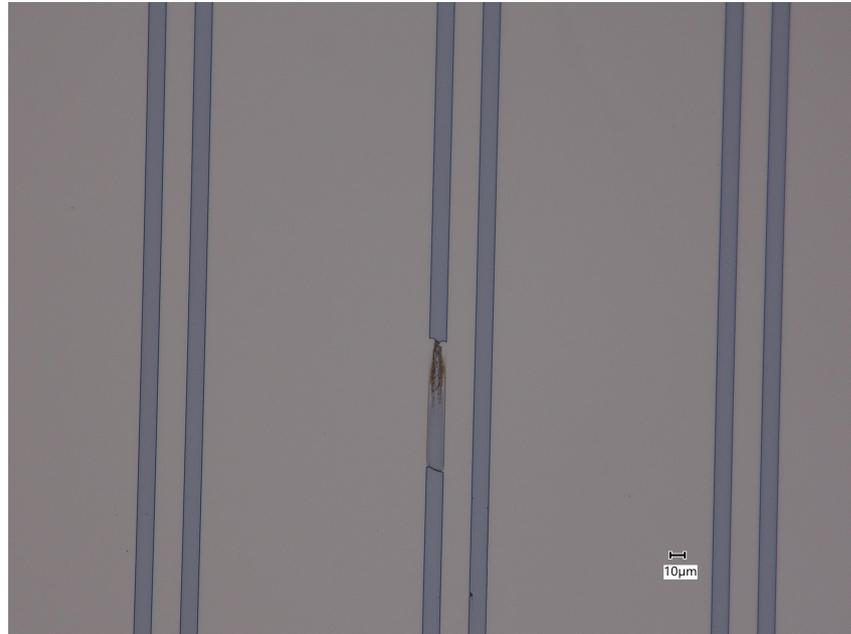
(c) Image of a short in the CPW. These type of defects were the most common for fabricated samples to turn out unusable. Most likely they were caused by bubbles or dirt in the photoresist.
