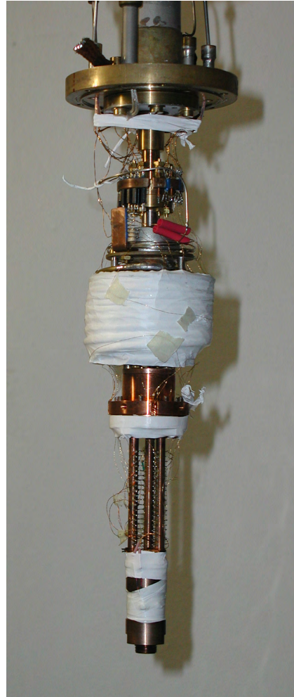
Figure 4.4: (a) Schematical drawing and (b) photograph of the dilution fridge unit. Heat exchangers in the condensation line: (1) spiral shaped heat exchanger with the ^4\text{He} bath, (2) Joule-Thomson heat exchanger with the main pumping line, (3) heat exchanger with distillation chamber and (4) counter flow heat exchanger with the diluted ^3\text{He} . (A), (B) flow impedances, (C) Degussit tubes, (D) sintered copper, (E) copper ring (both taken from [16]).
