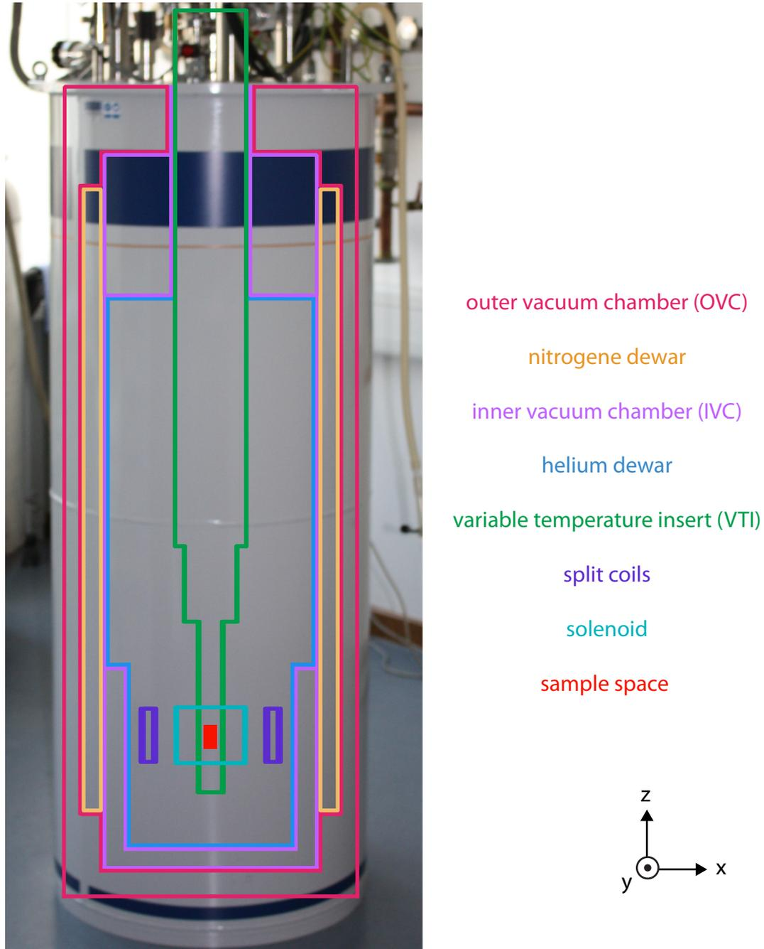
**Figure 6.1:** The "Chaos" cryostat (components see legend).
