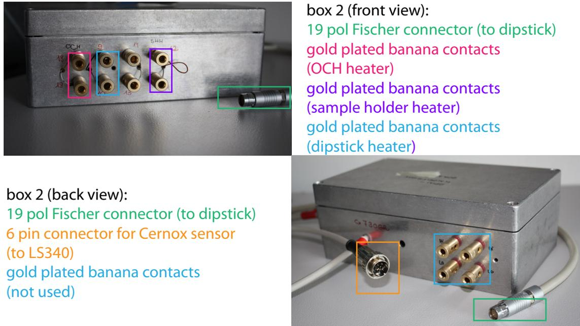
**Figure 6.5:** Measurement box 2 (components see legend).
