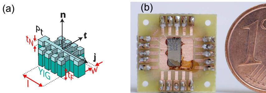
**Figure 2.6:** (a) Sketch of the Hall bar patterned YIG/Pt bilayer and definition of the coordinate system by  $\mathbf{j}$ ,  $\mathbf{t}$ , and  $\mathbf{n}$ . (b) Picture of a mounted and contacted YIG/Pt sample and a 1 Euro cent coin to serve as a rule. The photograph is provided by our former bachelor student Dominik Irber [111].
