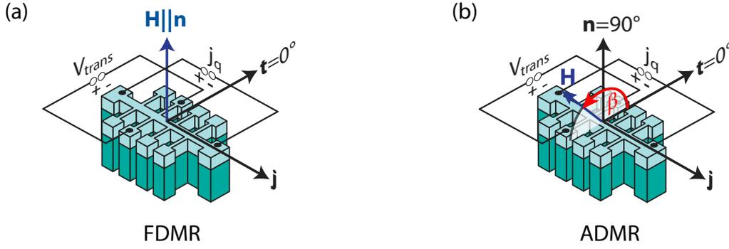
**Figure 3.3:** Measurement geometry for (a) field dependent magnetoresistance experiments (FDMR) at a fixed orientation of the external magnetic field ( $\mathbf{H} \parallel \mathbf{n}$ ) and (b) angle dependent magnetoresistance experiments (ADMR) in oopj configuration as defined in Sec. 2.2.2.
