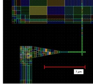
**Figure 4.9:** Short circuited ground planes. The structure equals the normal junction structures, only the Josephson junction itself is removed and a direct aluminium bridge is inserted.
