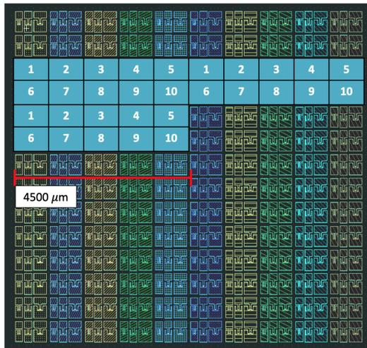
**Figure 4.1:** Early SQUID pattern in layout editor. The different colours of each column of the SQUID-triplets indicate different charge dose doses for the ground planes, the blue numbered boxes indicate different charge doses for the Josephson junctions
