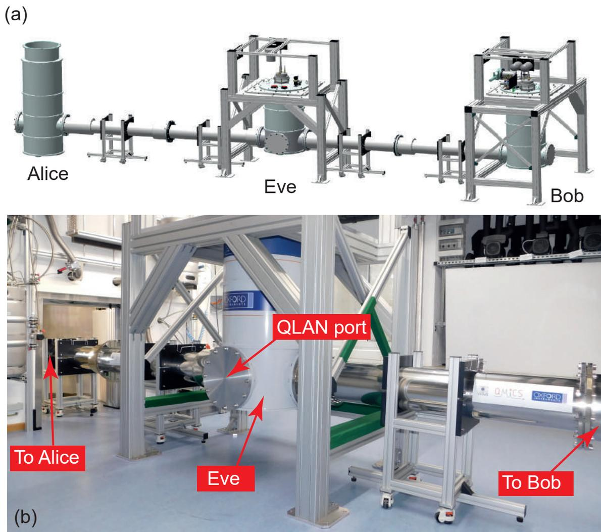
**Figure 7.2:** (a) CAD drawing of the cryogenic link and the OVC shields of Alice, Bob, and Eve. Image courtesy of Oxford Instruments. (b) Photograph of the installed cryogenic link, taken in the Eve lab. More details regarding a lab plan are provided in Fig. 7.5. The Eve cryostat is designed with four ports to enable potential connection of additional link arms. One of these ports, covered by a blind flange, is visible on the photograph (“QLAN port”).
