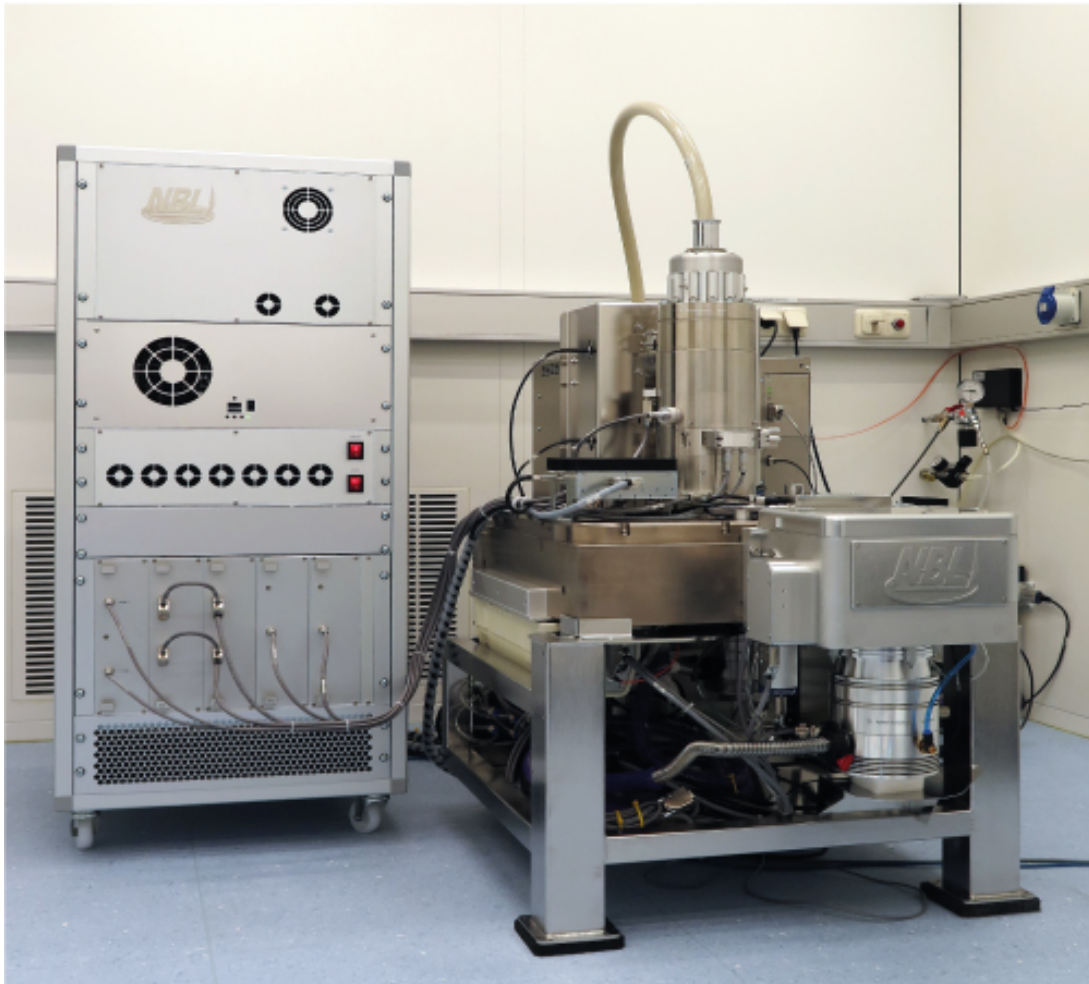
Figure 3.4: Photograph of the electron beam system nB5 from NanoBeam Limited.
