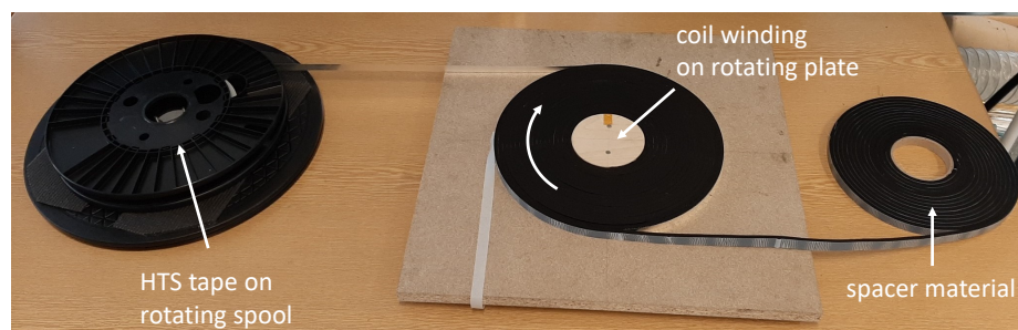
Figure 7.1: Home built setup for the fabrication of the HTS winding. The HTS tape and the spacer material are both wound simultaneously around the centerpiece by slowly turning the rotating plate.
