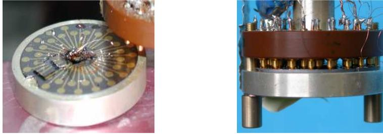
**Figure 4.6:** A wafer damaged by forces arising from different thermal expansion coefficients of the Si wafer and the silver ring (left) and the wafer mounting (right).
