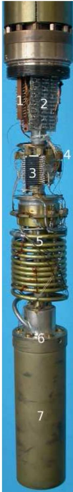
**Figure 4.3:** Photograph of the dilution unit. The thermal anchoring at 4 K (1), the RC-filter PCB (2), the connectors (3) and the thermal anchoring (4) at Joule-Thompson temperature, the still with the subsequent heat exchanger (5) ending in the mixing chamber (6), and the shielded sample stage (7) can be identified.
