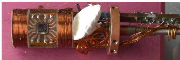
**Fig. 6.1:** 500 mK setup sample holder with a JJ mounted and bonded on a chip carrier printed circuit board (PCB). One observes the Helmholtz coil surrounding the PCB and the bonded sample. In the measurements a cryoperm or a brass pot protects the wiring and shields the sample.
