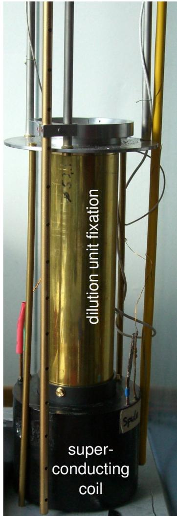
**Fig. 8.4:** A superconducting coil mounted in the dilution unit dewar setup. For the out-of-plane magnetization of the ferromagnetic interlayer of a SIFS  $\pi$ -junction in chapter 9, a commercially available superconducting coil is mounted in the dilution unit dewar setup.
