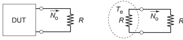
Figure C.2: The equivalent noise temperature T_e of an arbitrary white noise source, DUT.
